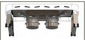
2. When powering with two EcoBurners, it is only possible to fit them in the Outer Spring Clip positions **(3)** as shown in the diagram above.
